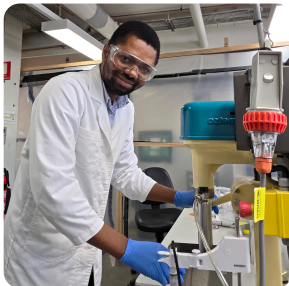
PhD Azeez Aregbe (UOM) using a Denver Cell for flotation experiments in the lab at UOM
