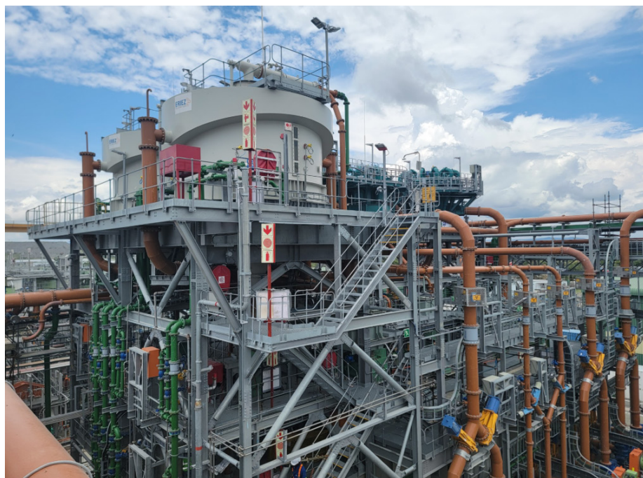
A HydroFloat CPF-300 installation - HydroFloat is an aerated fluidised-bed separator which combines the benefits of density separation with the selectivity of flotation
